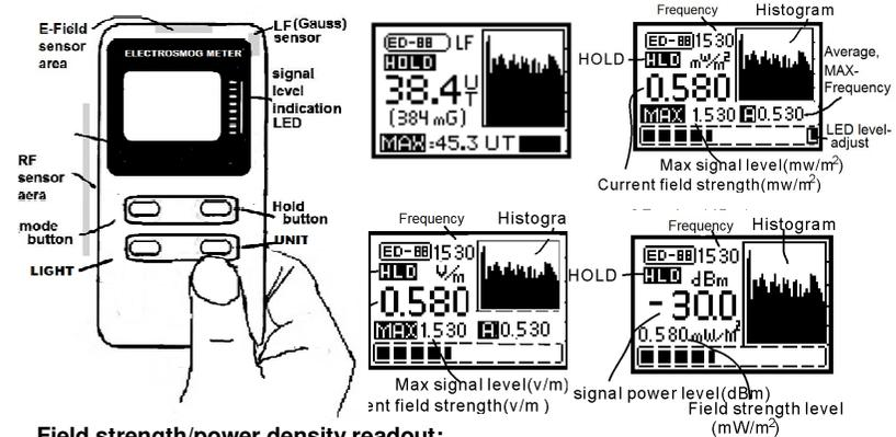
**Field strength/power density readout:**
